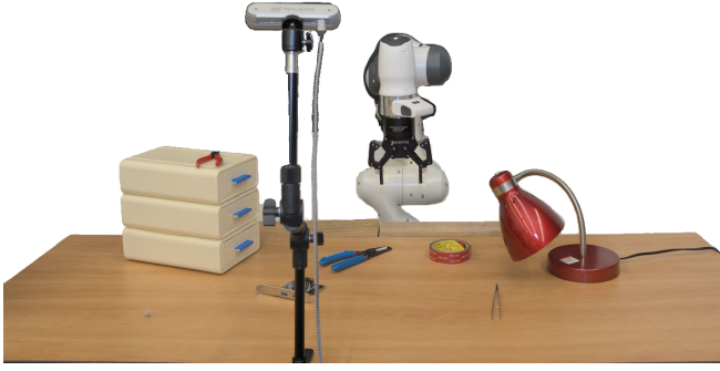
Fig. 5: Robot setup. A Franka Panda robot with a Robotiq Gripper. A RealSense D455 depth sensor captures the scene.
