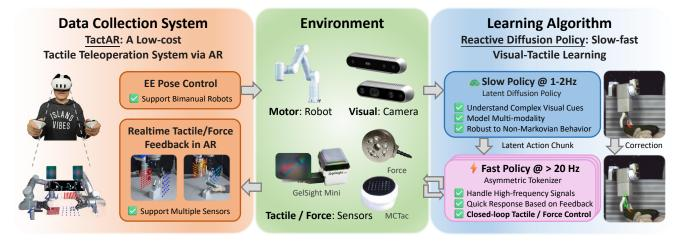
Fig. 1: **TactAR** is a low-cost and versatile teleoperation system which can provide real-time tactile / force feedback via Augmented Reality (AR). **Reactive Diffusion Policy (RDP)** is a slow-fast imitation learning algorithm that can model complex behaviors with a slow policy and achieve closed-loop control based on tactile / force feedback with a fast policy.
