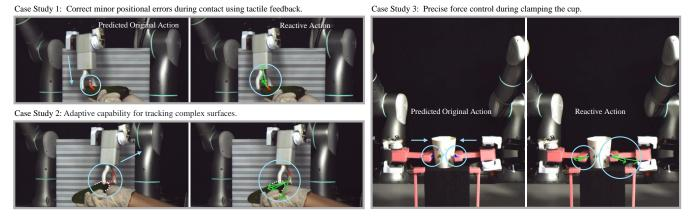
Fig. 13: Visualization of the RDP inference process. The red (left) and blue (right) dots can be seen as the predicted action chunk of the slow policy. The green arrow represents the correction direction and magnitude (scaled up for better visibility) of the reactive action predicted by the fast policy during inference. Please see the videos on the website for more details.
