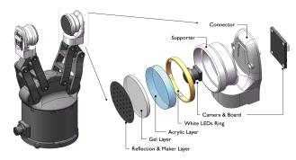
Fig. 10: Improved MCTac Sensor for our task. The left part is the gripper integrated illustration, and the right part is the detailed structure and components of the camera-based tactile sensor.
