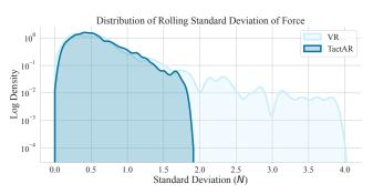
Fig. 15: The stability of contact forces with different teleoperation systems in *Peeling* task. Data collected with TactAR has higher stability of contact forces compared to traditional VR teleoperation.
