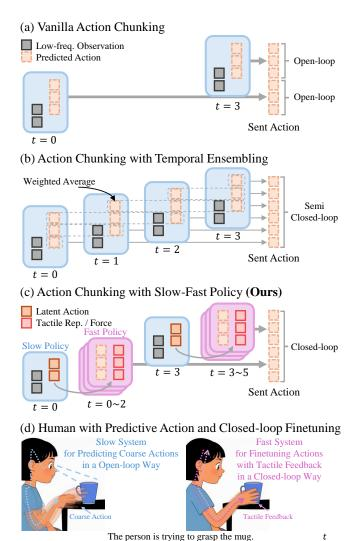
Fig. 9: Comparison among various pipelines. (a) Vanilla action chunking [2] with open-loop control during the chunk execution. (b) Action chunking enhanced with temporal ensembling [14, 21] for semi-closed-loop control. (c) Our slow-fast inference pipeline, showcasing closed-loop capabilities with fast responsive adjustments. (d) Human control patterns in contact-rich tasks.
