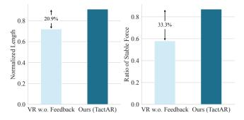
Fig. 6: Teleoperation data quality of 10 users on *Peeling* task (no perturb.) w./w.o. tactile / force feedback.
