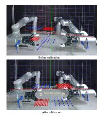
Fig. 8: Calibration process in AR. The user adjust the translation and rotation of the virtual coordinate system such that it can align with the pre-defined TCP position (the white sphere) and the origin of the world coordinate system.
