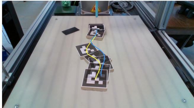
Fig. 1: Overlay of snapshots from one of the cameras, showing dynamic feedback linearization in action on the setup. The reference trajectory is shown in blue, while the executed path is yellow.
