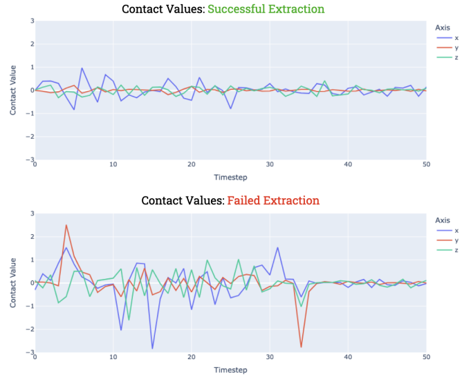
Fig. 7. Sample contact values in the x, y, and z-axes measured during both successful and failed extractions. Values are far more erratic in cases where the extraction is unsuccessful.
