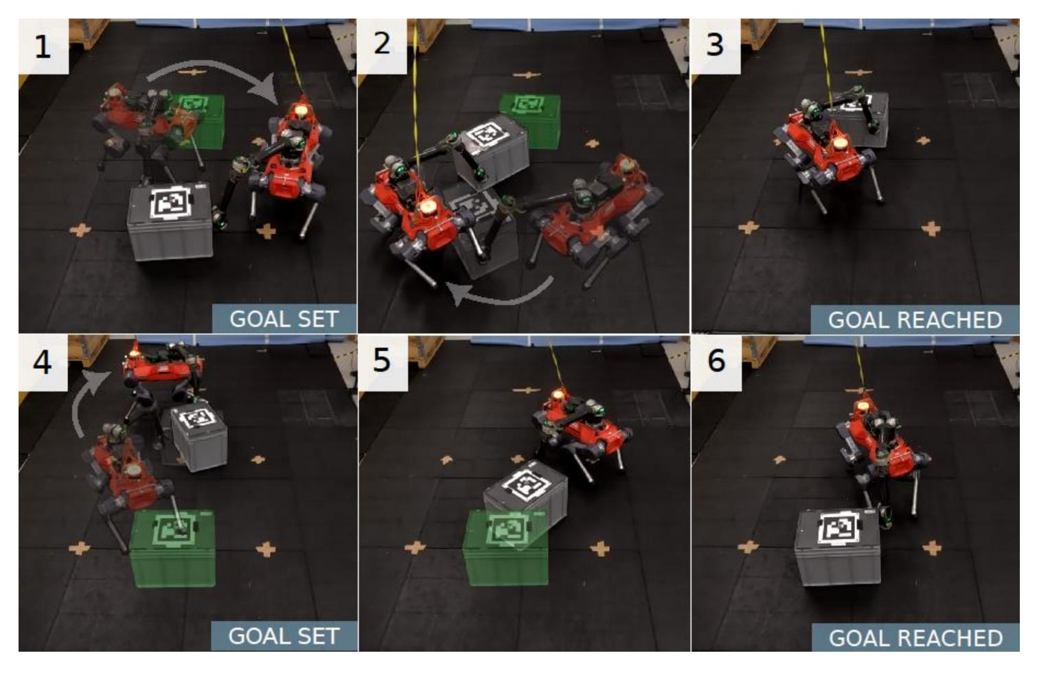
**Robustness with object of different material (Plastic,** Cardboard, Wood), shape (CUboid, CYlinder) and size
